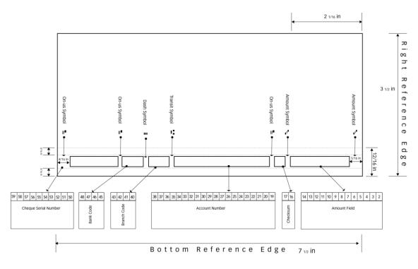
Figure5: MICR line encoding locations and details (as in Annexure V)
